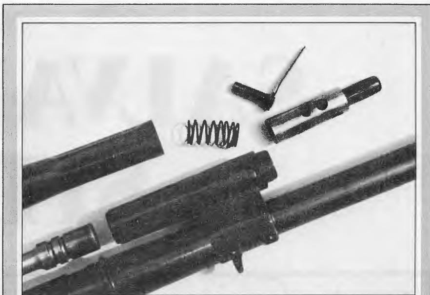
Type 74 gas system, disassembled.
